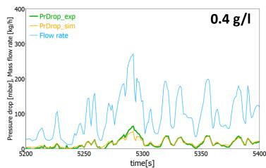
The model is able to accurately predict deltaP for filters at both soot-free and soot loaded conditions
