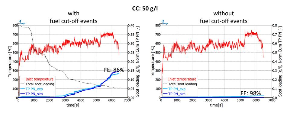
By deactivation of fuel-cut off mode the GPF retains its high filtration efficiency
